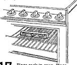
Place rack in oven. Place level on rack, first side to side; then front to back. If range is not level at the front, adjust the leveling legs up or down until the range is level. If rear of range needs adjusting, adjust rear leveling legs up or down until range is level. If rear legs are adjusted downward more than 1/8", add shims under anti-tip bracket. Replace front panel.
